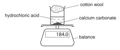
The beaker was placed on a balance and the mass of the beaker and contents recorded every minute.
