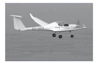
This aeroplane has an electric motor powered by fuel cells.
