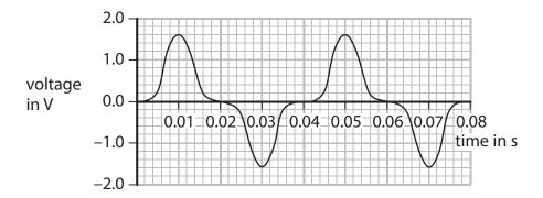
State the maximum output voltage of the dynamo.
