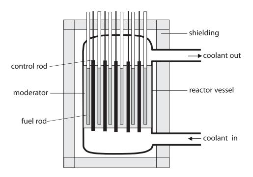
(a) Describe nuclear fission and how the chain reaction is controlled.
