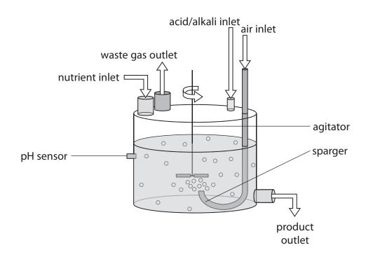
(a) An acid or alkali can flow through the acid/alkali inlet to maintain a constant pH within the fermenter.
