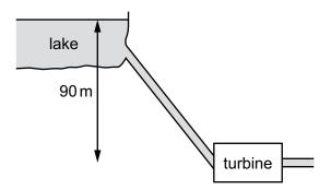
The mass flow rate of the water is  $2400 \text{ kg min}^{-1}$ . The turbine has an efficiency of 75%.
