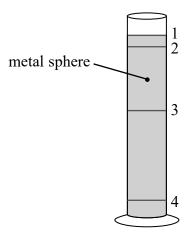
9 Elastic bands are placed around the cylinder in the positions 1, 2, 3 and 4 as shown. The time taken for the sphere to fall between two of the elastic bands is going to be recorded.
