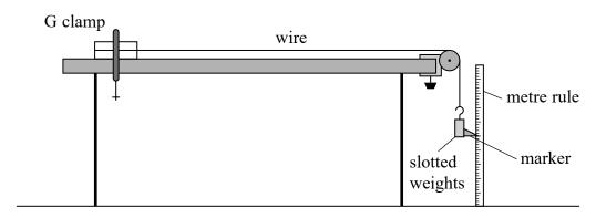
The initial length of the wire was measured. Slotted weights of known values were added to the hanger at the free end of the wire. Each time a weight was added, the new position of the marker was read from the metre rule and the extension calculated.
