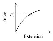
The point marked  $\times$  is the elastic limit of the wire.
