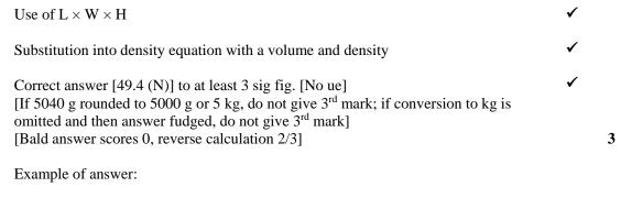
$80 \text{ cm} \times 50 \text{ cm} \times 1.8 \text{ cm} = 7200 \text{ cm}^3$   $7200 \text{ cm}^3 \times 0.70 \text{ g cm}^{-3} = 5040 \text{ g}$   $5040 \times 10^{-3} \text{ kg} \times 9.81 \text{ N/kg}$ = 49.4 N
