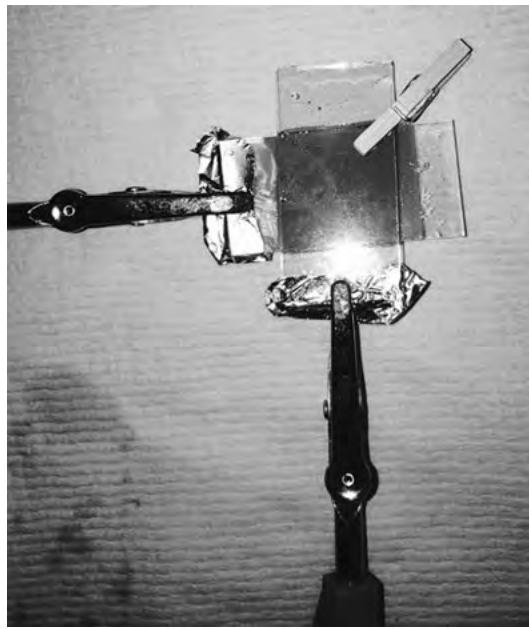
When measured with a high resistance voltmeter, the e.m.f. is found to be 400 mV. When the solar cell is connected across a  $4700\ \Omega$  resistor, the potential difference across the resistor is 18 mV.
