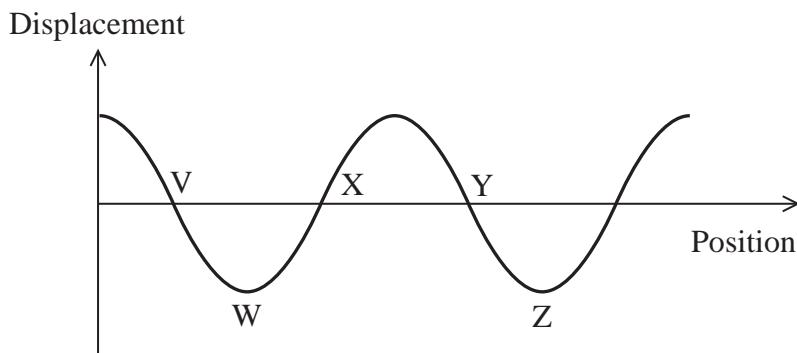
Which of the following could show the positions of a pair of particles moving in the same direction at that instant?
