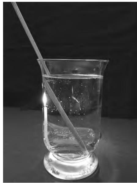
When the vase is full of water, the stick appears to be broken and the candle appears distorted because of refraction.
