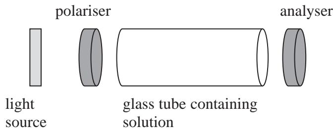
An experiment led to the conclusion that the solution had rotated the plane of polarisation of the light by  $35^\circ$ .
