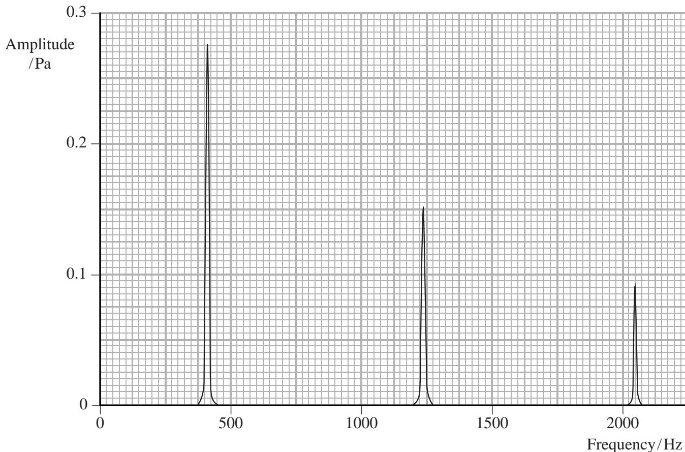
Several frequencies of sound are observed. Each frequency corresponds to a different standing wave in the tube. The loudest, at 410 Hz, is the fundamental frequency. The higher frequencies observed are known as overtones.
