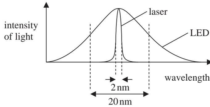
Light of different wavelengths will travel at different speeds along the fibre.
