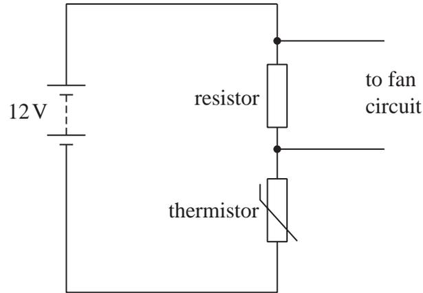
Calculate the resistance of the resistor.
