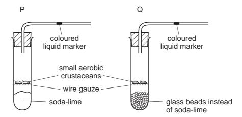
Which way does the liquid marker move?
