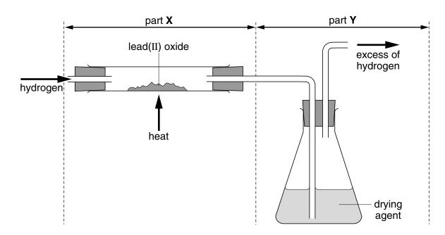
**16** Lead(II) oxide is reduced in the apparatus shown.
