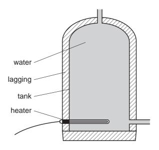
What is the main process by which heat moves through the water?
