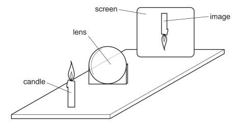
Various focused images are produced on the screen by moving the lens and the screen backwards and forwards.
