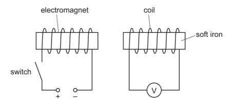
The switch is closed. The electromagnet magnetises quickly.
