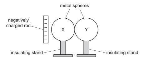
Using the insulating stand, sphere Y is moved away from sphere X.
