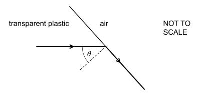
The ray of light enters the air travelling parallel to the surface of the plastic.
